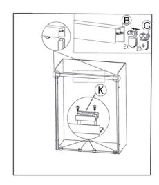
Before putting top profiles onto wall channels, pls insert the wheels as per showed picture. Then fix the plastic parts onto the bottom profile.
