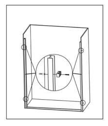
4. Fix the wall chanells with supplied plugs and screws.
