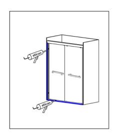
You now need to seal the enclosure with a good anti fungal silicone, only seal the out side of the enclosure. DO NOT SEAL THE ENCLOSURE ON BOTH SIDES!
