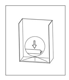
3. Put the bottom profile on the floor.
