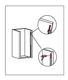
Ensure that you use a spirit level to make sure that the wall channel is completely plumb before you mark and drill the holes.
