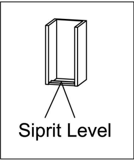
1. Ensure that the floor/tray is level before you begin with the installation.
