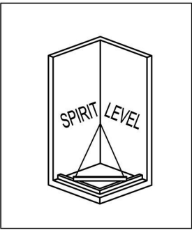
1. Ensure that the floor/tray is level before you begin with the stallation.
